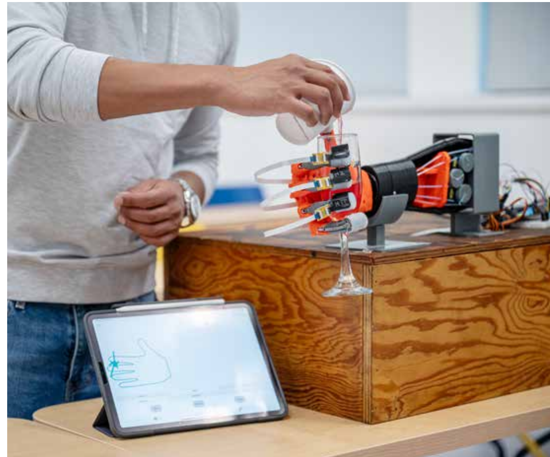
UBC engineers collaborated with Frontier Robotics, Honda's research institute, to develop a soft sensor "skin" for applications in robotics and prosthetics. Photo: UBC Applied Science/Paul Joseph
